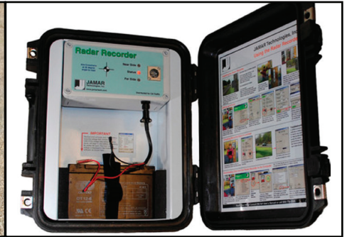
Radar Recorder Units
